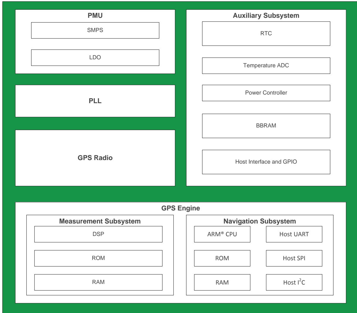
FIGURE 2 – SiRFstarIV™ GSD4e GPS SoC BLOCK DIAGRAM
