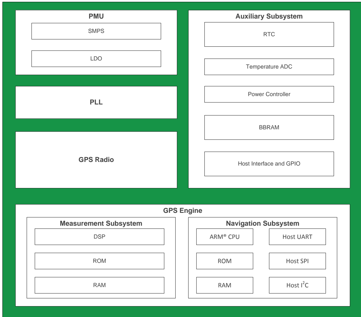
FIGURE 2 – SiRFstarIV™ GSD4e GPS SoC BLOCK DIAGRAM
