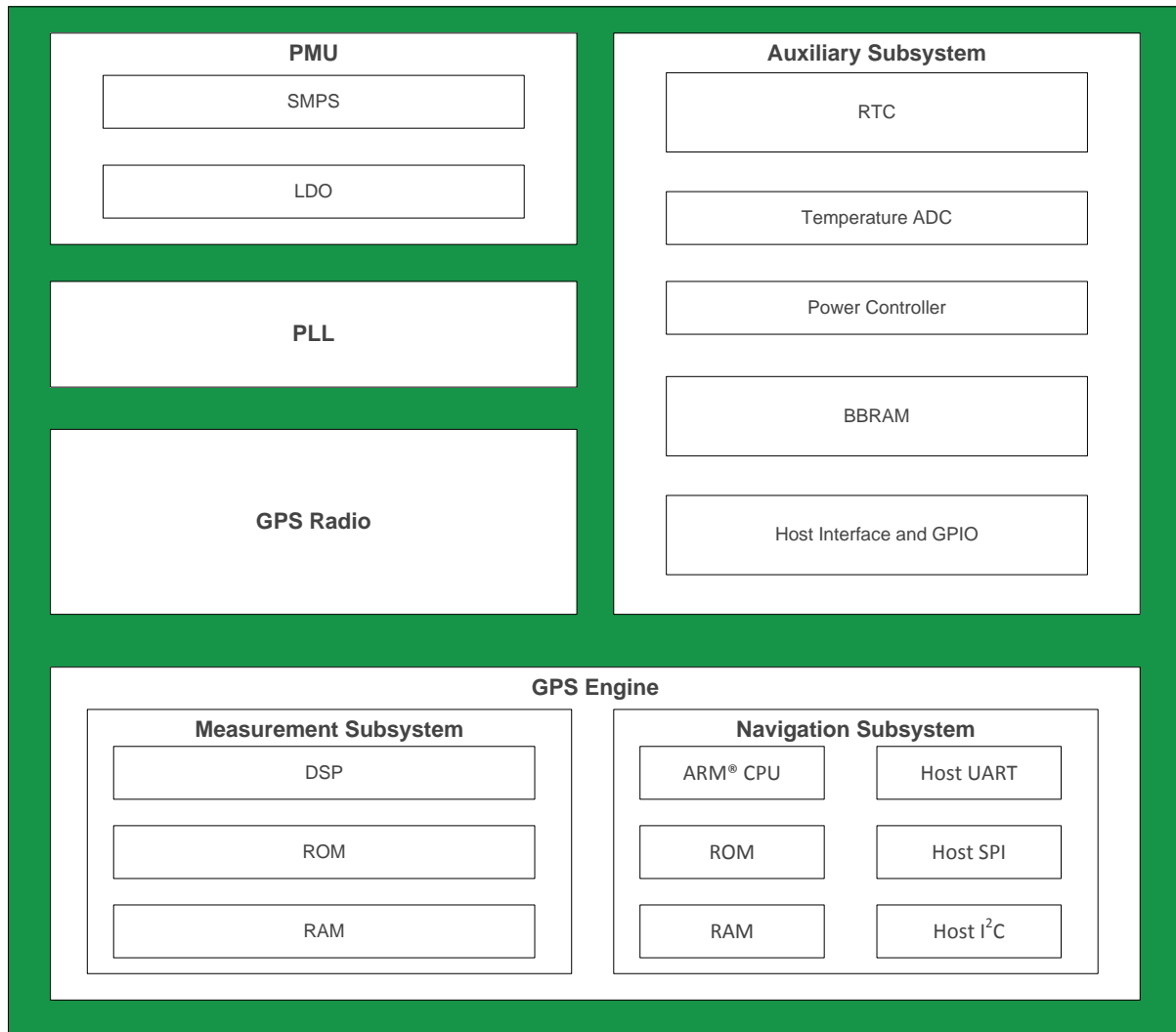
FIGURE 2 – SiRFstarIV™ GSD4e GPS SoC BLOCK DIAGRAM
