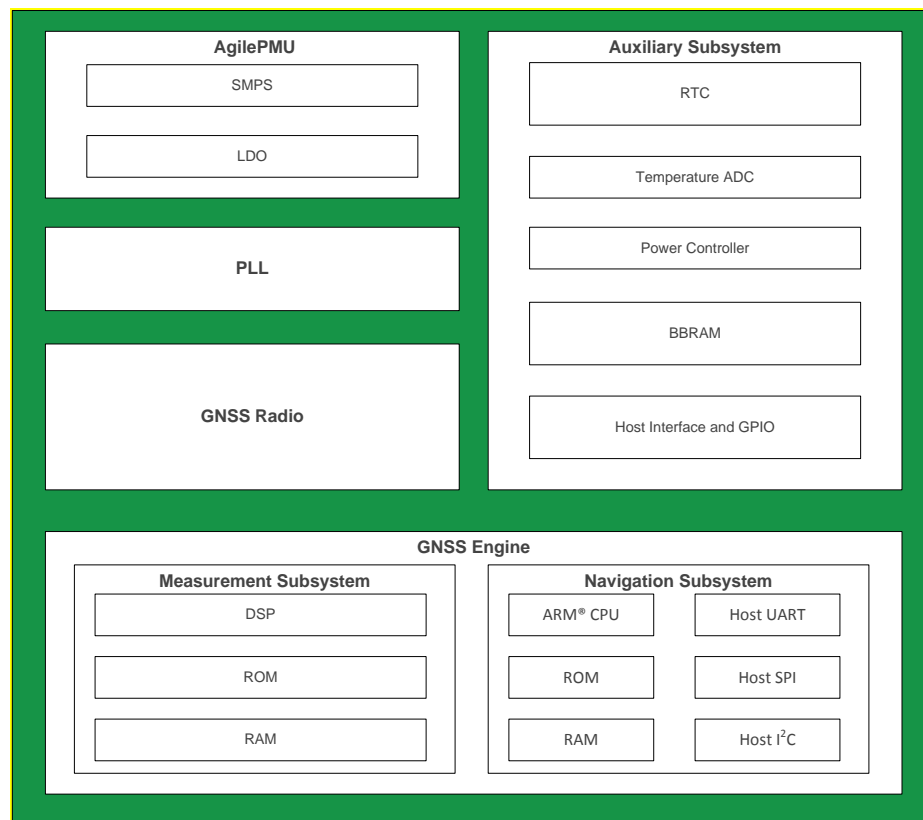
FIGURE 2 – SiRFstarV™ 5e GNSS SoC BLOCK DIAGRAM
