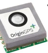
Additionally, the Nano Hornet module combines OriginGPS' proprietary low-profile GPS antenna with a dual-stage LNA, RF LDO, SAW filter, TCXO, RTC crystal and RF shield with market-leading SiRFstarIV™ GPS SoC.
