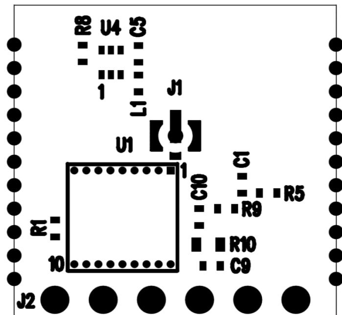
FIGURE 7 - INTERFACE ADAPTOR BOARD COMPONENTS PLACEMENT
