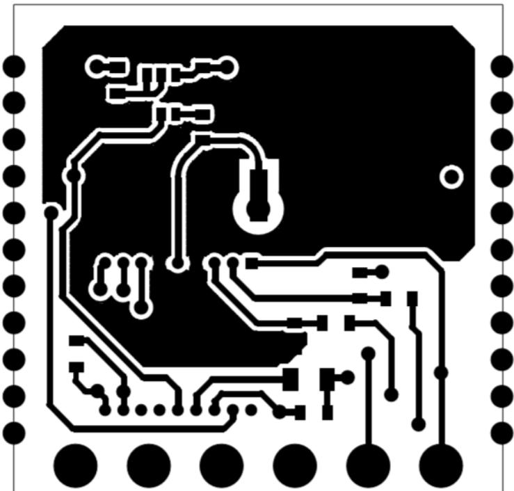
FIGURE 9 - INTERFACE ADAPTOR BOARD TOP LAYER ROUTING
