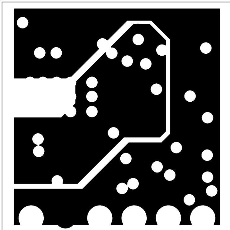
FIGURE 11 - INTERFACE ADAPTOR INNER LAYER 2 ROUTING
