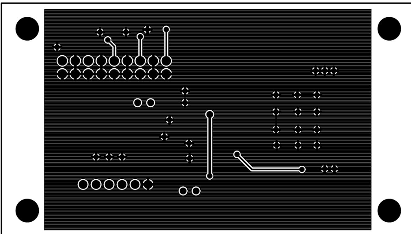
FIGURE 6 – MAIN BOARD BOTTOM LAYER ROUTING
