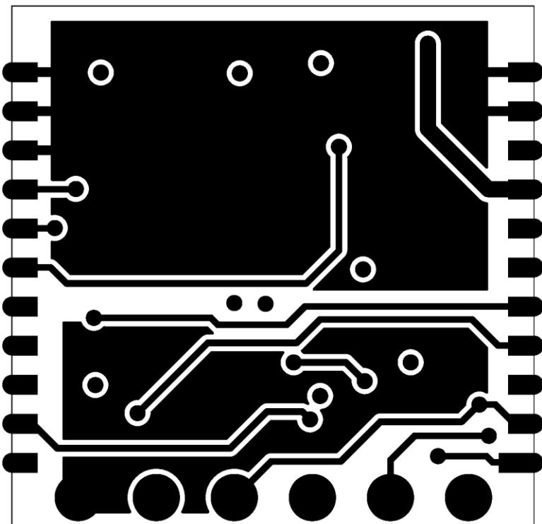
FIGURE 12 - INTERFACE ADAPTOR BOTTOM LAYER ROUTING
