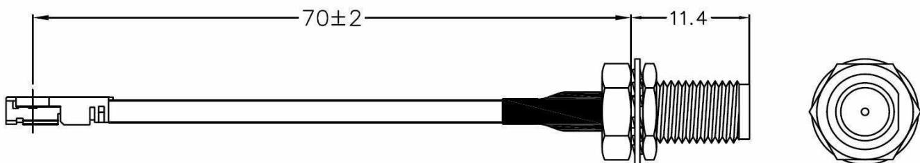
FIGURE 19 - I-PEX MHFIII TO SMA-TYPE ADAPTOR MECHANICAL OUTLINE
