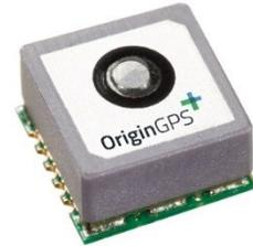
Additionally, the ORG1510-MK module combines OriginGPS' proprietary low-profile GNSS antenna with a dual-stage LNA, RF LDO, SAW filter, TCXO, RTC crystal and RF shield.
