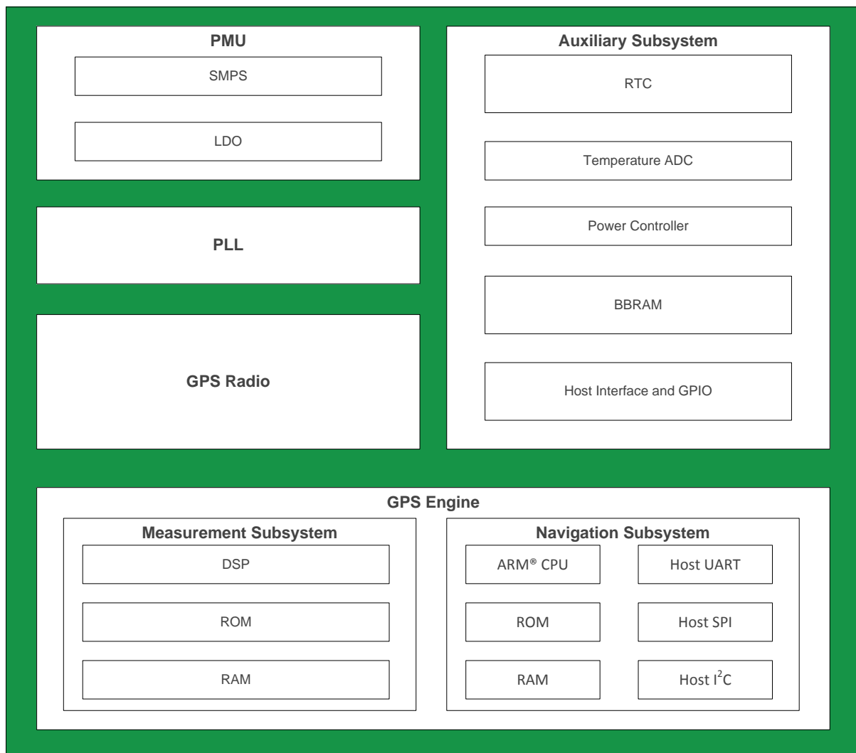
FIGURE 2 – SiRFstarIV™ GSD4e GPS SoC BLOCK DIAGRAM
