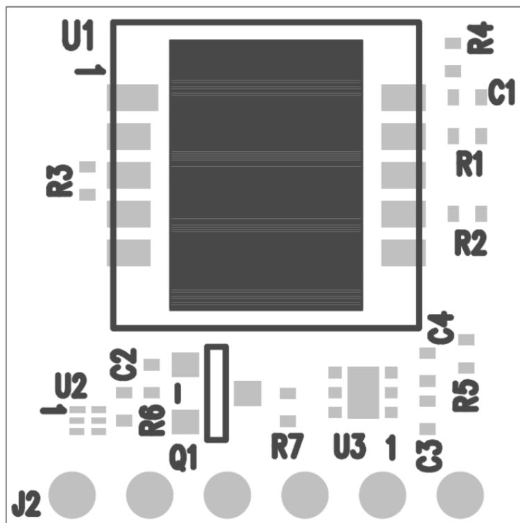
FIGURE 7 - INTERFACE ADAPTOR BOARD COMPONENTS PLACEMENT
