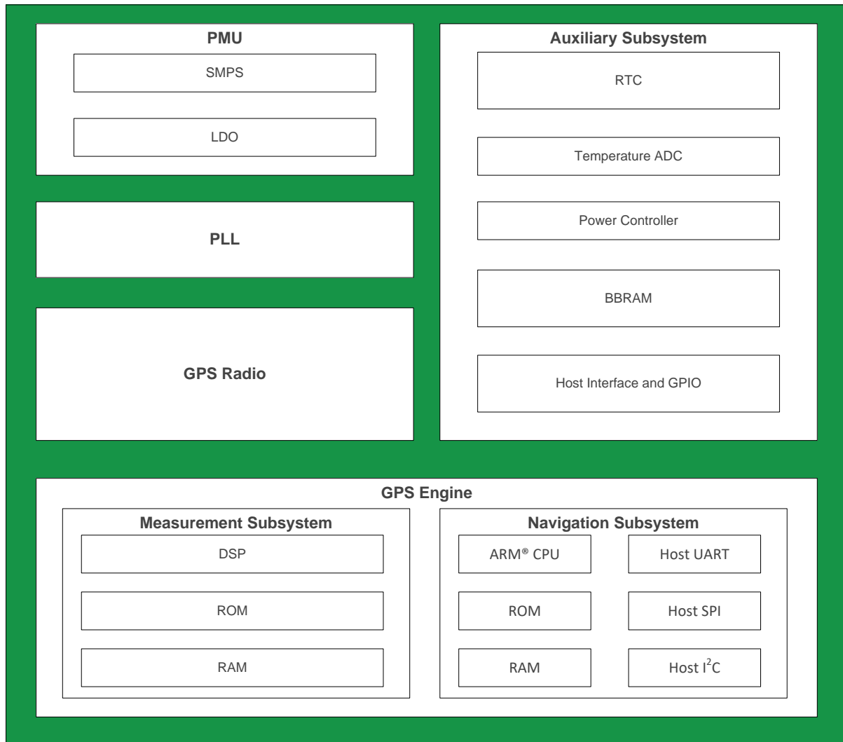
FIGURE 2 – SiRFstarIV™ GSD4e GPS SoC BLOCK DIAGRAM
