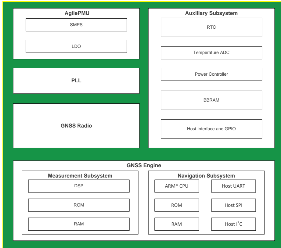
FIGURE 2 – SiRFstarV™ 5e GNSS SoC BLOCK DIAGRAM
