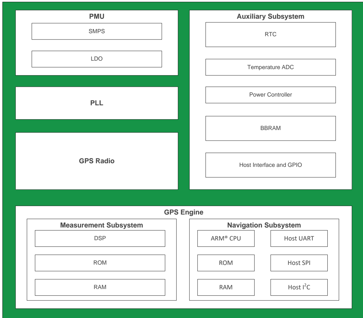
FIGURE 2 – SiRFstarIV™ GSD4e GPS SoC BLOCK DIAGRAM
