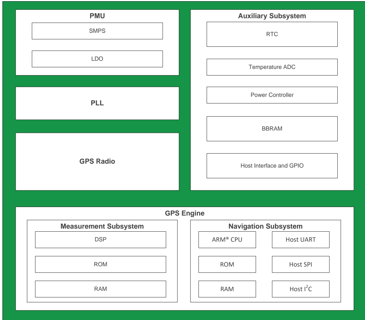
FIGURE 2 – SiRFstarIV™ GSD4e GPS SoC BLOCK DIAGRAM
