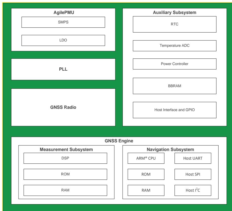
FIGURE 2 – SiRFstarV™ 5e GNSS SoC BLOCK DIAGRAM
