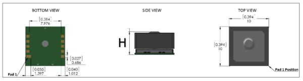
Figure 7. Mechanical Layout
