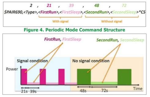
Figure 5. Periodic Mode - Time Parameters
