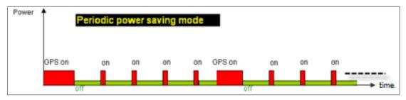
Figure 3. Periodic Mode - Power Consumption
