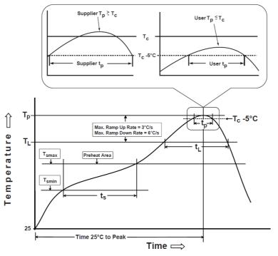
Figure 10. Recommended Soldering Profile
