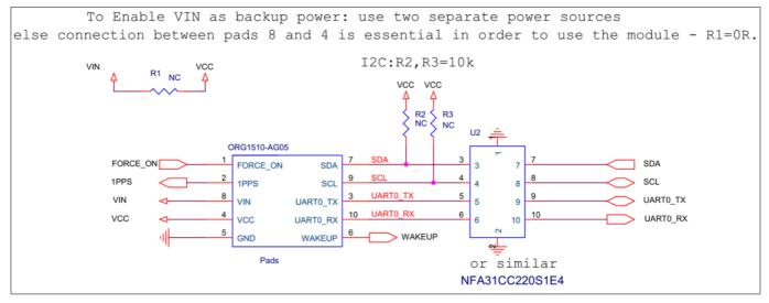
Figure 9. ORG1511-AG05 Module – Reference Schematic Diagram
