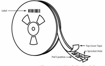
Figure 11. Module Position
